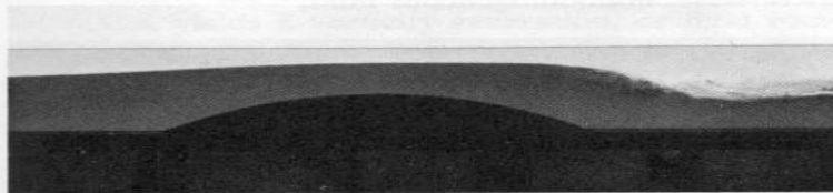
15. Hydraulic drop in a two-fluid system. Note the increase of thickness of the upper fluid downstream.
