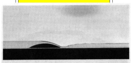
5. Hydraulic jump at a water surface. The approach Froude number is less than one.
