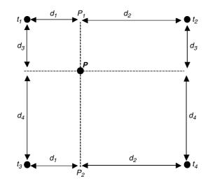
Figure 2. Illustration of bilinear interpolation of the PRISM data. *P* is the location for prediction;  $t_1, t_2, t_3$ , and  $t_4$  are the values of climate variables at the centers of the four neighboring PRISM tiles;  $d_1, d_2, d_3$ , and  $d_4$  are the relative spatial distances.  $P_1$  and  $P_2$  are predictions based on simple linear interpolations of the climate variable values  $t_1$  and  $t_2$ , and  $t_3$  and  $t_4$ , respectively
