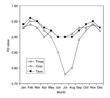
Figure 5. Values of  $R^2$  for polynomial functions modeling monthly maximum ( $T_{max}$ ), minimum ( $T_{min}$ ) and mean ( $T_{ave}$ ) temperatures of PRISM data using geographic variables including latitude, longitude, elevation, and their transformations and combinations
