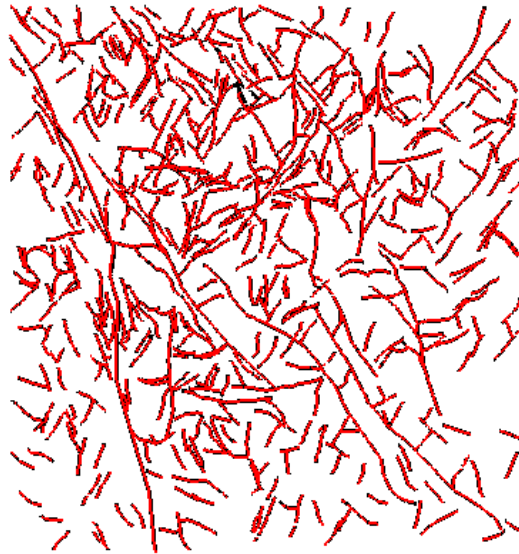
Fig. 7. Comparison of input traces to an inspection plane of a single realization of the Canadian Shield DFN model cut on the same plane as input traces.
