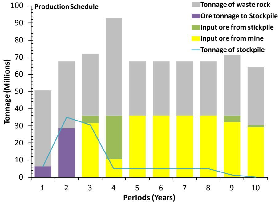
Figure 1: Production schedule using OK block model with a stockpile.
