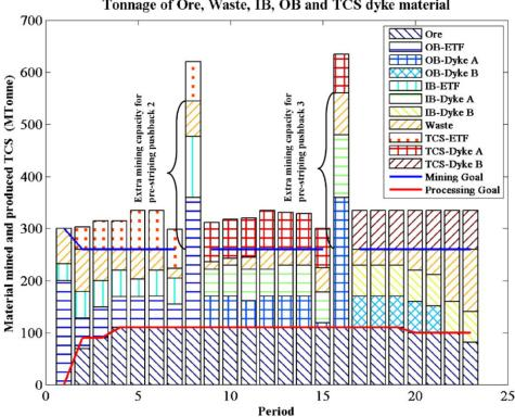
Tonnage of Ore, Waste, IB, OB and TCS dyke material
