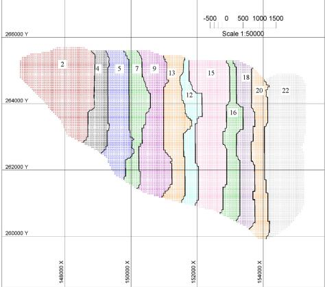
Figure 11: Mining sequence on level 302.5 m for Scenario 2b
