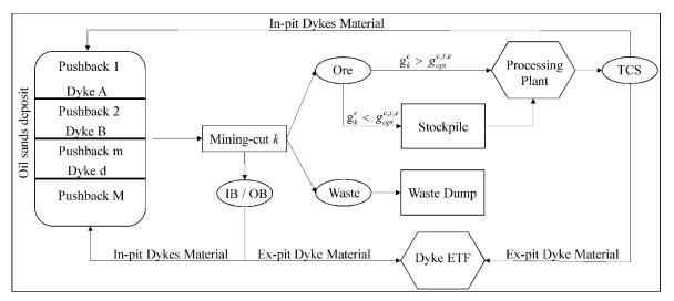
Figure 1: Material flow for oil sands production planning and waste management modified after Ben-Awuah et al. (2012)
