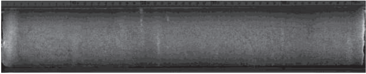
Figure 3. The Ice Core Image from the Line Scanner – our starting point for image processing. The top of the core (depth = 0), is on the left. The bottom of the core (depth = 51.5 cm) is on the right.
