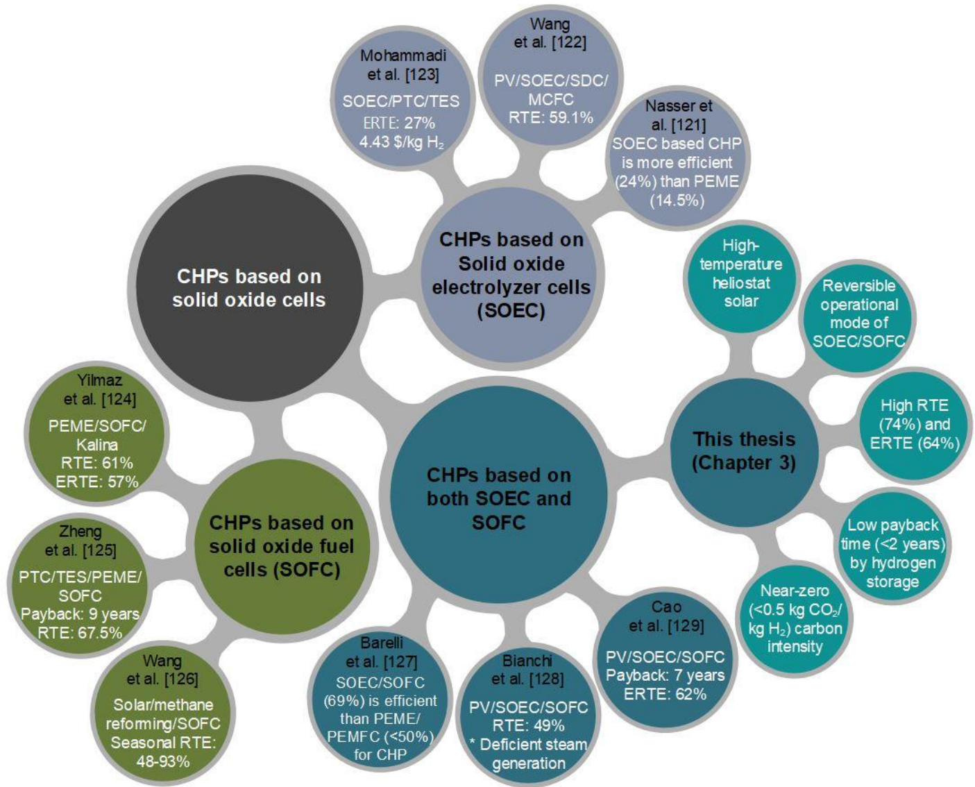
Figure 1.12: Graphical literature review about the use of SOEC, SOFC, or combined SOEC and SOFC for hydrogen production/usage and presentation of the novelties of this study. SOEC: Solid oxide electrolyzer cell; SOFC: Solid oxide fuel cell; PEME: Proton exchange membrane electrolyzer; PTC: Parabolic trough collector; TES: Thermal energy storage; SDC: Solar dish collector; RTE: Round-trip efficiency; ERTE: Exergy round-trip efficiency.
