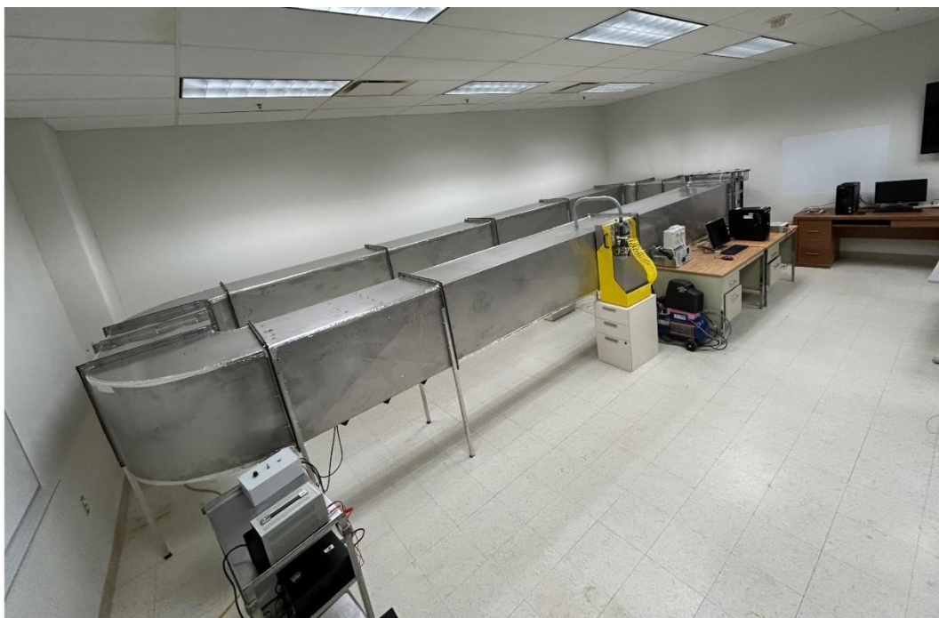
Fig. 6.4. Experimental setup for evaluating filtration efficiency and pressure drop.
