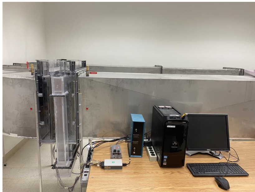
Fig. 6.6. Experimental setup for evaluating heat transfer and energy performance of the disinfection unit accommodated in the wind tunnel.
