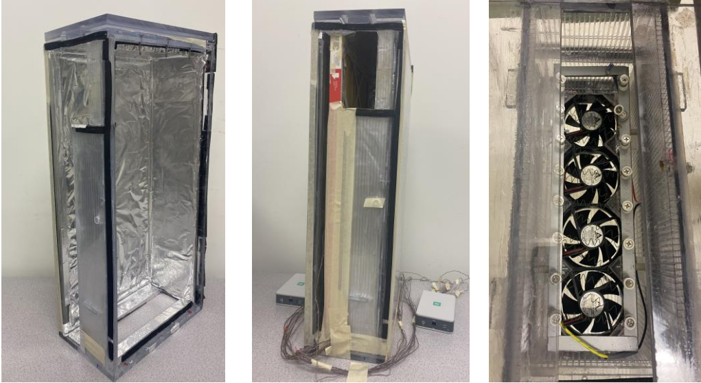
Fig. 6.5. Manufactured prototype for thermal disinfection of the two-stage filtration systems.
