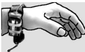
Figure 1: The prototype system and kinematic hand model. Bend \angle A = \angle B = 1.5\angle C \propto v (metacarpal to fingertip image distance)
